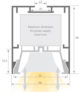
System with front removable tray which permits easy access to the led strip and power supply, therefore allowing very fast and simple maintenance of the electrical installation
